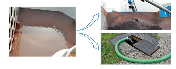
The **solid dehydrated part** is brought by the conveyors system directly to the bins provided by the client, while the **liquid part** is sent to the discharge drain.
