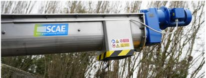
The **sludge** is extracted directly from the tank or from the sludge thickener, conditioned with suitable **polymer** and separated silently and efficiently.
